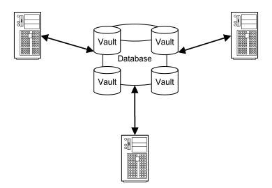
Figure 6 - Data Integration Model 4: Partitioned Warehouse
