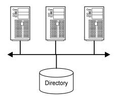
Figure 4 - Data Integration Model 2c: Facilitated Peer to Peer
