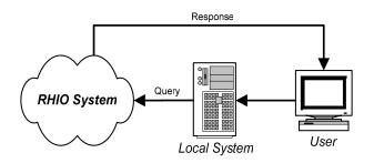
Figure 10 - Application Integration Model 3: Direct User Access through a Local Application
